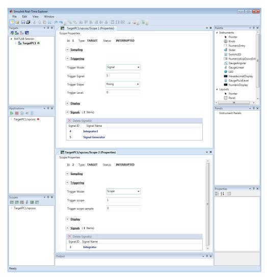
9 Start both **Scope 1** and **Scope 2** ( on the toolbar). You must explicitly start and stop both scopes.
