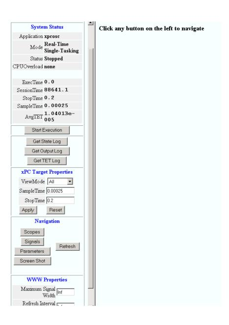
**Note:** The **ViewMode** control is visible in the **Simulink Real-Time Properties** pane only if you add two or more scopes to the target computer.
