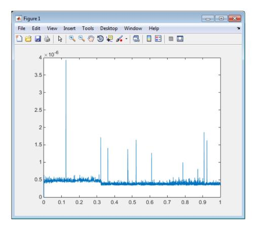
The TET is the time to calculate the signal values for the model during each sample interval. If you have subsystems that run only under certain circumstances, plotting the TET shows when subsystems were executed and the additional CPU time required for those executions.
