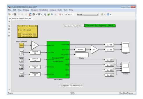
This generated model contains a masked subsystem with the same name as the subsystem in the Simulink FPGA domain model. Although the appearance is similar, this subsystem does not contain the Simulink algorithm. Instead, the algorithm is implemented in an FPGA bitstream. You reference and load this algorithm into the FPGA from this subsystem.
