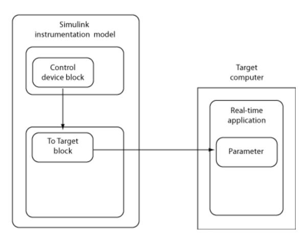
This block is implemented as a MATLAB S-function. The block is optimized so that it only changes a parameter on the real-time application when the input value differs from the value that existed at the last time step. This block uses the parameter downloading feature of the Simulink Real-Time command-line interface. This block is available from the slrtlib/Displays and Logging block sublibrary. See To Target for further configuration details.
