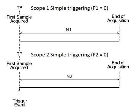
• sc(2).TriggerSample = ts > 0 — Scope 2 triggers ts samples after Scope 1 is triggered. Trigger point TP2 for Scope 2 is ts samples after TP1 for Scope 1.
