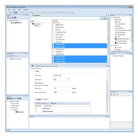
The software creates a log file named SCOPE1\_1.DAT and writes data to that file. When the size of SCOPE1\_1.DAT reaches 4096 bytes (the value of Max write file size), the software closes SCOPE1\_1.DAT and creates SCOPE1\_2.DAT, SCOPE1\_3.DAT, and so on until it fills the last log file, SCOPE1\_9.DAT. If the real-time application continues to collect data after the software closes SCOPE1\_9.DAT,
