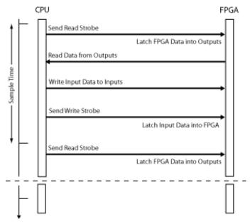
• Coprocessing — blocking — The CPU and the FPGA run synchronized and in tandem. When the FPGA execution time is short compared to the Speedgoat target machine sample time, and you want the FPGA to complete before the model continues, select this coprocessor mode.
