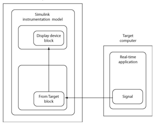
Because only one numerical value per signal is uploaded during a time step, the number of samples of a scope object is set to 1. The block uses the capability of the Simulink Real-Time command-line interface and is implemented as a MATLAB S-function. This block is available from the slrtlib/Displays and Logging sublibrary. See From Target for further configuration details.
