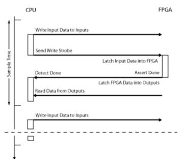
• Coprocessing — nonblocking with delay — The CPU and the FPGA run synchronized and in tandem. When the FPGA execution time is long compared to the Speedgoat target machine sample time, select this coprocessor mode. For example, you could select this mode to manage multiple FPGAs effectively in parallel.
