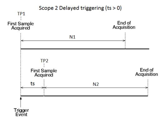
Setting sc(2). TriggerSample to a value ts larger than (N + P - 1) does not cause an error. It implies that Scope 2 cannot be triggered, because Scope 1 cannot acquire more than (N + P - 1) samples after TP.
